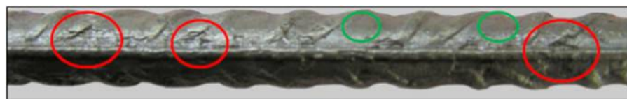
Notes: Embedded specimen with mass loss 4.06 percent. Green cycle: non corroded area and red cycle: spots of localized corrosion that leads to severe pit corrosion
